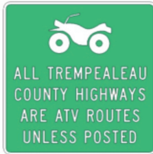
36" x 36" when used on state highways. Smaller sizes may be used on local roads. D11-10A (white on green) or R59-52 (black on white)
